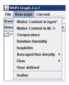
This menu allows you to create a new diagram page for the selected quantity. When you select a menu item, WUFIGraph displays a diagram of the building component where you can determine the region over which the selected quantity shall be averaged. Of course, only those quantities can be selected which WUFI2D has written to the result file (see the "Computational Parameters" dialog of WUFI2D).
