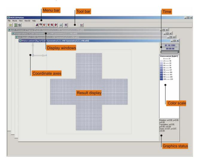
The main window contains several document windows, each of which shows one of the computed quantities (e.g. temperature, moisture content etc.) as a two-dimensional color-coded field superimposed on the component geometry. You can rotate the diagrams into a side view so that, in addition to the color coding, the values of the fields are also visualized by their heights along the z-axis. Start the Movie display to see an animation of the hygrothermal processes in the component.
