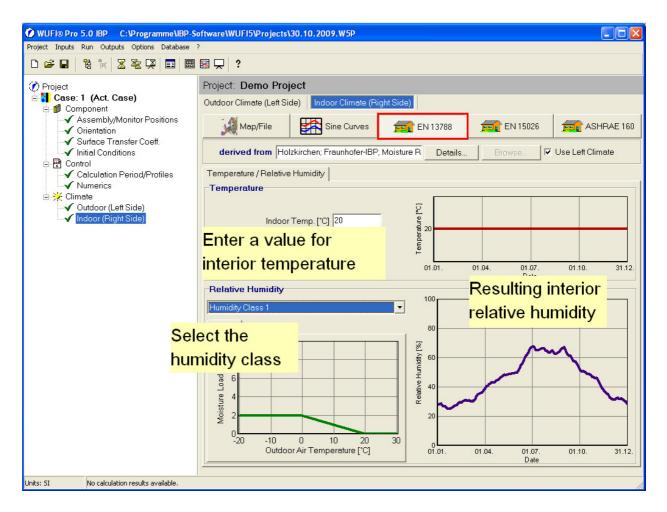
Normally the moisture load in residential buildings should be less than 4 g/m<sup>3</sup> - this corresponds to humidity class 1 or 2. The values for humidity classes 3 and 4 are very high and should only be used if it has been established that in the investigated case the moisture load is indeed extremely high. They are not appropriate for normal residential buildings.
