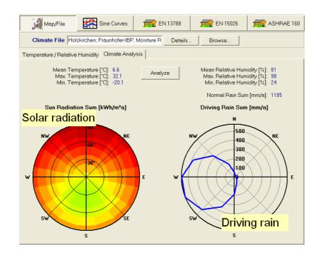
The rain rose shows the yearly driving rain sum on vertical surfaces for different orientations. The scale of this diagram is adapted to accommodate the maximum driving rain load occurring at this location. The amount of driving rain is given in mm/year.
