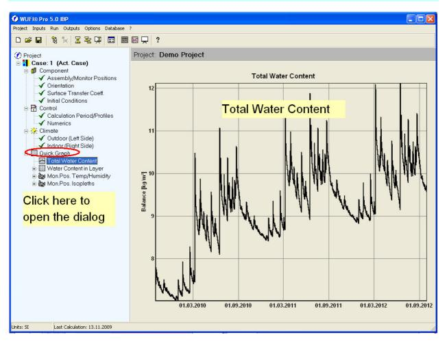
Usually, the main criterion for assessing the results is the behaviour of the total water content. It shows whether moisture has accumulated or dried out during the investigated period.
